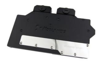
The Koolance VID-NX980 is a full coverage video block for water cooling NVIDIA reference GeForce GTX 980 cards in single and multi video card configurations. It utilizes a high-performance microfin (0.5mm) design made of solid copper with anti-corrosive nickel plating. Fitting threading is standard G 1/4 BSPP. For multiple card configurations, video connectors are also available.
