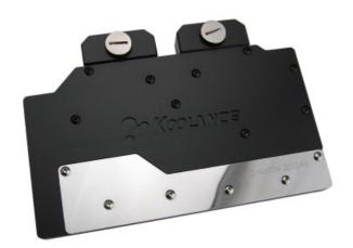
The Koolance VID-NXTTN2 is a full coverage video block for water cooling NVIDIA reference GeForce GTX TITAN, TITAN Black, GTX 780, and GTX 780 Ti cards in single and multi video card configurations. It utilizes a high-performance microfin (0.5mm) design made of solid copper with anti-corrosive nickel plating. An aluminum back plate is included to handle the rear memory chips.
