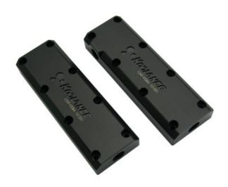
Koolance video bridge connectors link multiple video water blocks together with ease. CNT-VDB4 is for combining four (dual L-bracket) video blocks in consecutive PCI-Express slots. This version uses a combination serial+parallel flow path to minimize pressure drop. This product is only compatible with Koolance VID-series water blocks which have detachable fitting bases (launched in 2013 or later).
