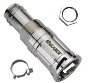
Koolance patented quick disconnect coupling with automatic shutoff. 10mm (3/8in) ID female panel-mountable hose barb with clamp. It will only fit a Koolance VL2 male quick disconnect.
