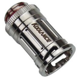
Koolance patented quick disconnect coupling with automatic shutoff. G 1/4 BSPP (parallel) thread female fitting for screwing directly into a water block or other component. It will only fit a Koolance VL2 male quick disconnect.
