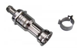
Koolance patented quick disconnect no-spill coupling with automatic shutoff. 6mm (1/4in) ID female panel-mountable hose barb with clamp. It will only fit a Koolance VL2N male quick disconnect.
