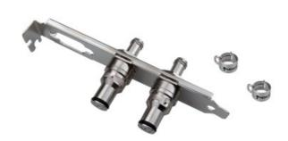
Koolance quick disconnect no-spill couplings with L-bracket. Fittings feature hose barbs on the inside for 6mm (1/4in) ID tubing and VL2N male fittings on the outside (for connection with female VL2N). The quick-disconnects enable the convenient connection and disconnection of external devices such as a Koolance Exos. The fittings are nickel-plated brass.
