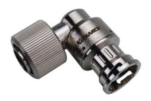
Koolance patented quick disconnect coupling with automatic shutoff. 13mm (1/2in) ID female swiveling elbow connection with compression fitting. It will only fit a Koolance VL3 male quick disconnect.
