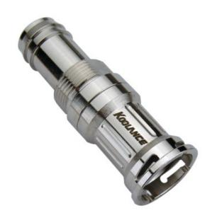
Koolance patented quick disconnect coupling with automatic shutoff. 13mm (1/2in) ID female panel-mountable barb fitting with spring clamp. It will only fit a Koolance VL3 male quick disconnect.
