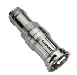
Koolance patented quick disconnect coupling with automatic shutoff. 13mm (1/2in) ID female panel-mountable hose barb with clamp. It will only fit a Koolance VL3 male quick disconnect.
