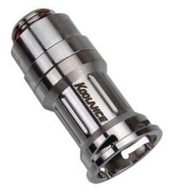
Koolance patented quick disconnect coupling with automatic shutoff. G 1/4 BSPP (parallel) thread female fitting for screwing directly into a water block or other component. It will only fit a Koolance VL3 male quick disconnect.
