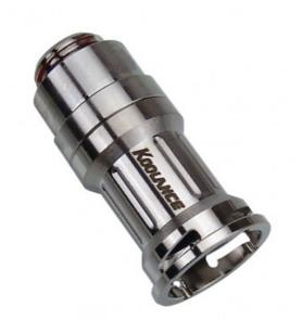
Koolance patented quick disconnect coupling with automatic shutoff. G 1/4 BSPP (parallel) thread female fitting for screwing directly into a water block or other component. It will only fit a Koolance VL3 male quick disconnect.
