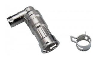
Koolance patented quick disconnect no-spill coupling with automatic shutoff. 13mm (1/2in) ID female swiveling elbow connection with hose barb and clamp. It will only fit a Koolance VL3N male quick disconnect.
