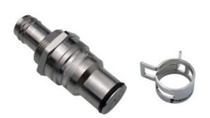
Koolance patented quick disconnect no-spill coupling with automatic shutoff. 13mm (1/2in) ID male panel-mountable hose barb with clamp. It will only fit a Koolance VL3N female quick disconnect.
