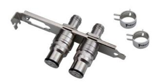
Koolance quick disconnect no-spill couplings with L-bracket. Fittings feature barb fittings on the inside for ID 10mm (3/8in) tubing and VL3N male fittings on the outside (for connection with female VL3N). The quick-disconnects enable the convenient connection and disconnection of external devices such as a Koolance Exos. The fittings are nickel-plated brass.
