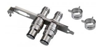
Koolance quick disconnect no-spill couplings with L-bracket. Fittings feature hose barbs on the inside for ID 13mm (1/2in) tubing and VL3N male fittings on the outside (for connection with female VL3N). The quick-disconnects enable the convenient connection and disconnection of external devices such as a Koolance Exos. The fittings are nickel-plated brass.
