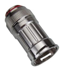
Koolance patented quick disconnect coupling with automatic shutoff. G 3/8 BSPP (parallel) thread female fitting for screwing directly into a water block or other component of same threading. It will only fit a Koolance VL4 male quick disconnect.
