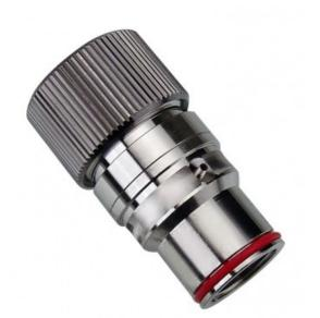
Koolance patented quick disconnect coupling with automatic shutoff. 13mm (1/2in) ID, 19mm (3/4in) OD male straight connection with compression fitting. It will only fit a Koolance VL4 female quick disconnect.
