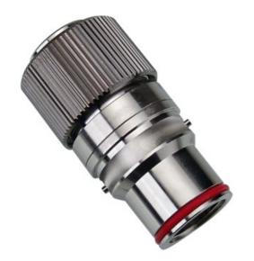
Koolance patented quick disconnect coupling with automatic shutoff. 16mm (5/8in) ID, 19mm (3/4in) OD male straight connection with compression fitting. It will only fit a Koolance VL4 female quick disconnect.
