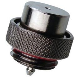
The VLV-VL002K safety valve releases built-up air pressure in situations such as corrosion, thermal expansion, etc. (at approximately 0.3-0.4kg/cm2, 4.3-5.7psi). G 1/4 BSPP thread.
