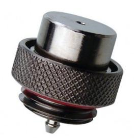
The VLV-VL002K safety valve releases built-up air pressure in situations such as corrosion, thermal expansion, etc. (at approximately 0.3-0.4kg/cm2, 4.3-5.7psi). G 1/4 BSPP thread.
