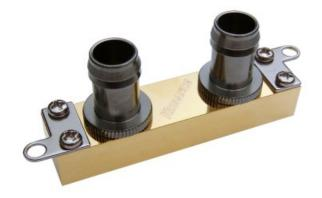
The VR-AS39 is a cooler for ASUS motherboard MOSFETbased voltage regulator circuits. It works with the 75mm (3") mounting hole distance. The VR-AS39 is created from solid copper and plated in gold. G 1/4 BSPP fitting threading.
