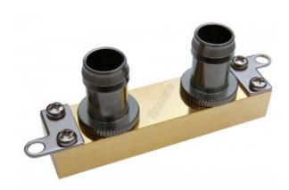
The VR-AS39 is a cooler for ASUS motherboard MOSFET-based voltage regulator circuits. It works with the 75mm (3") mounting hole distance. The VR-AS39 is created from solid copper and plated in gold. G 1/4 BSPP fitting threading.
