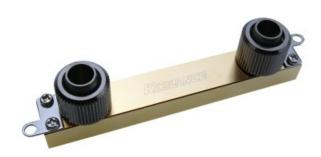
The VR-AS41 is a cooler for ASUS motherboard MOSFET-based voltage regulator circuits. It works with the 118mm (4.65") mounting hole distance. The VR-AS41 is created from solid copper and plated in gold. G 1/4 BSPP fitting threading.
