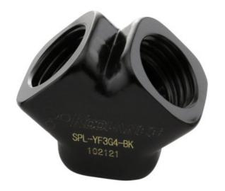
Koolance "Y-shape" tubing splitter with three female G 1/4 BSPP threads. Made of brass.
